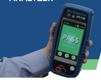
Simplify your wire harness testing. The DIT-MCO HT-128 provides a superior solution for point-to-point continuity analysis. These lightweight, handheld units can serve your diagnostic needs from product development and benchtop testing through field support and maintenance.
